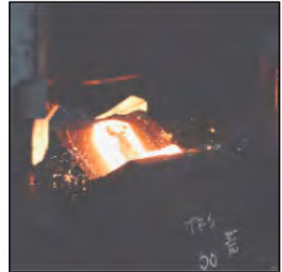
Forging. Three times forged in two forging dies shapes the billet into the raw forge.
