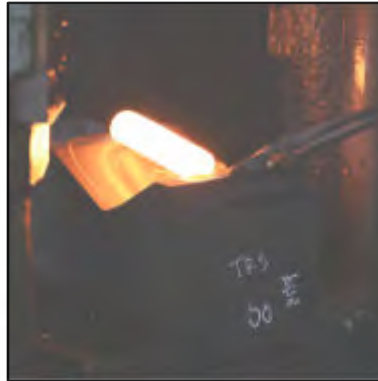
Cutting and heating of the billets and feeding them to the forge.
