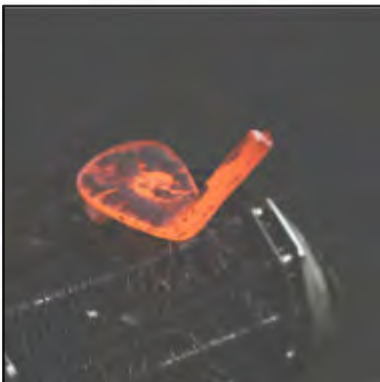
Removing excessive material and cooling down the raw forgings.
