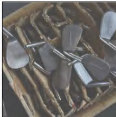
First grind and drilling the hosel.
