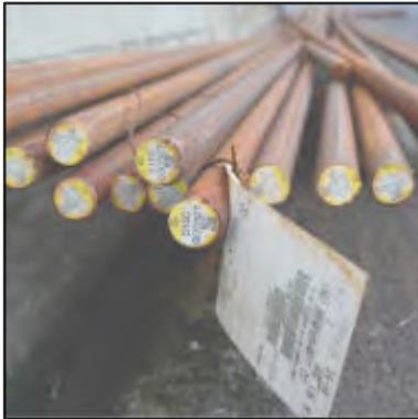
Raw Material Selection. Most used steel for forging is JIS S15C - S25C
