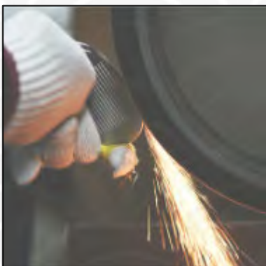
Shaping and grinding of the club head.
