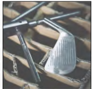
Consolidation forging and pressing of the grooves. Second grinding process.
